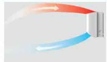
Hot air is drawn in from the top and cool air is discharged from the bottom to facilitate cool air showering down over the entire area.
